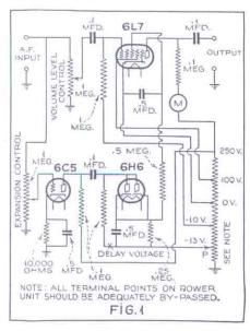
The input signal is applied to both the 6L7 and to a 6C5 amplifier simultaneously. The output of the 6C5 is rectified in the 6H6, providing a positive voltage with respect to the reference on the voltage divider. This bias signal is applied to the other input grid of the 6L7, where it produces an initial large negative bias. Under normal sound, the amplification factor of the
